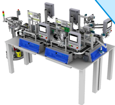
Modul Palettentransfersystem Cyber Physical System Plug and Produce
